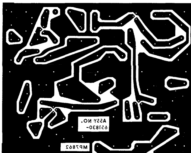
D. WIRING ON BACK OF BOARD A2 (VIEWED THROUGH FRONT)
